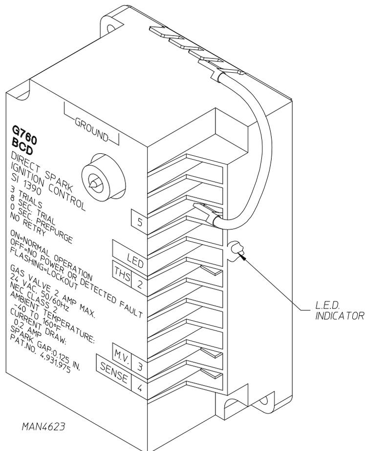
3. For Direct Spark Ignition (DSI) System Models Manufactured With ADC Module Part No. 882627
