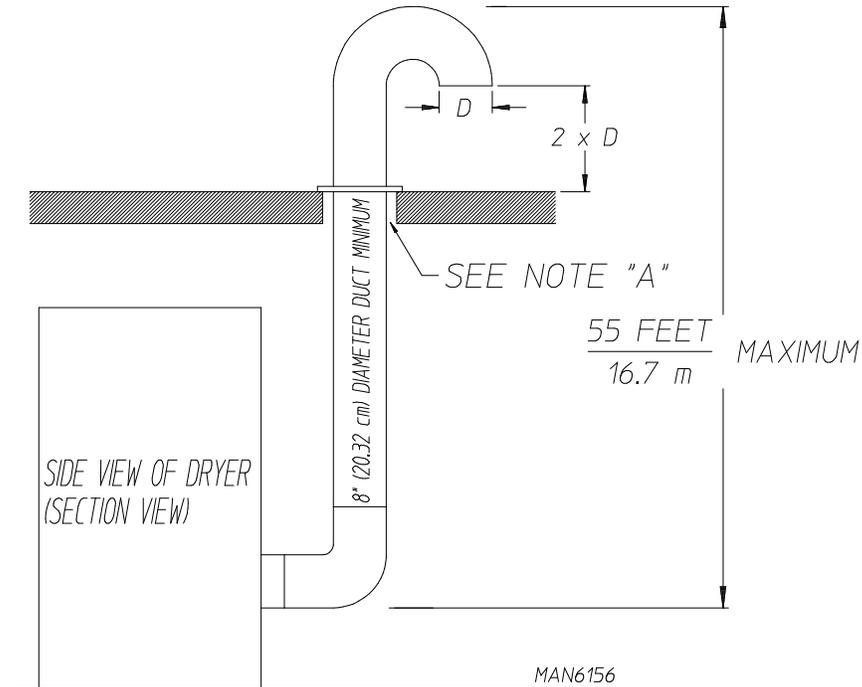
NOTE A: OPENING MUST BE TWO (2) INCHES (5.08 cm) LARGER THAN THE DUCT
