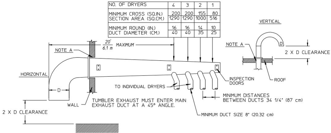
IMPORTANT: NO MORE THAN 4 DRYERS CAN BE CONNECTED TO ONE COMMON DUCT ( VENT ).
