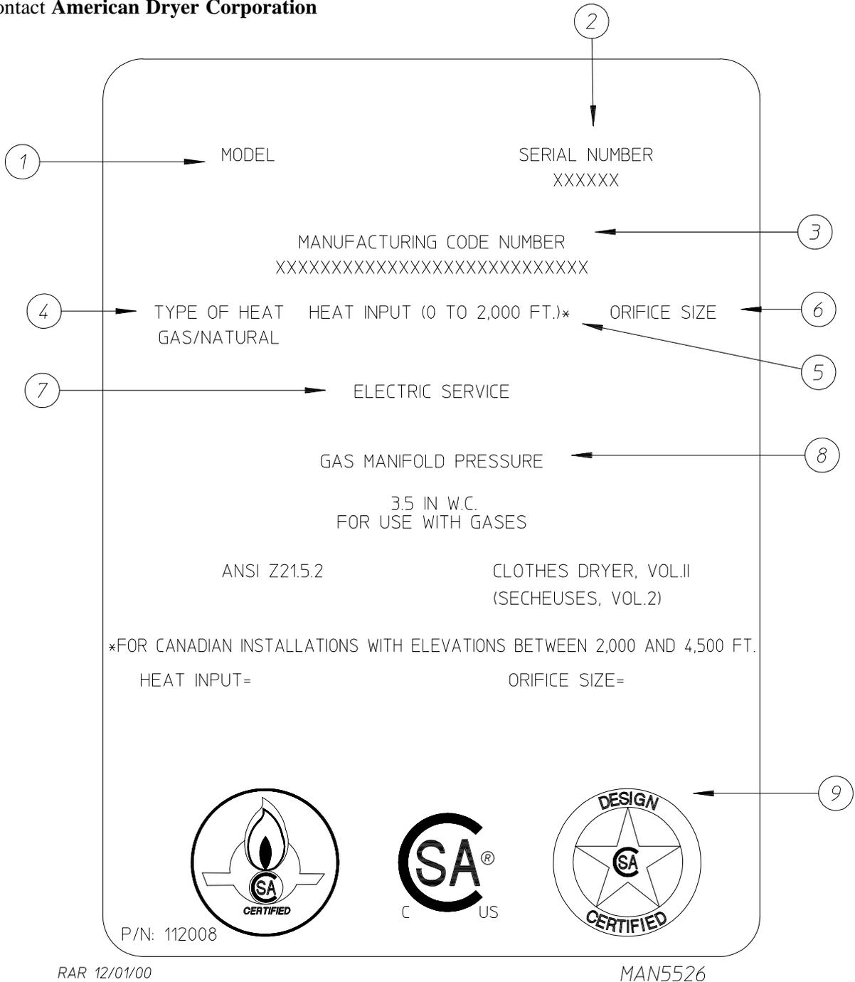
When contacting **American Dryer Corporation** certain information is required to insure proper service/parts information from **ADC**. This information is on the data label affixed to the left side panel area behind the top control (access) door. When contacting **ADC** please have the **model number** and **serial number** available.
